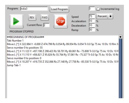
Note that the gripper is connected to Servo 0 and a zero value is its closed position and 55 is its open position. So, in the above program the robot will move almost directly to its right and pickup and object, move back to its rest position and open servo. Then it repeats.
