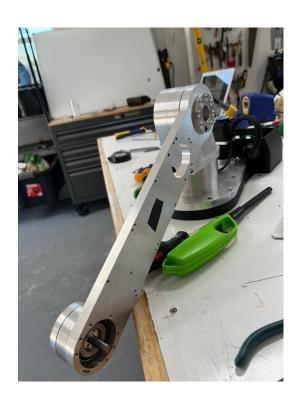
Note that the J2 ARM is not a symmetrical piece. In the above picture the entire arm was pressed onto the bearings backwards. This cost a significant amount of rework and clever use of various sockets and the shop press. Two people were required to hold robot and operate the press while undoing the mistake.
