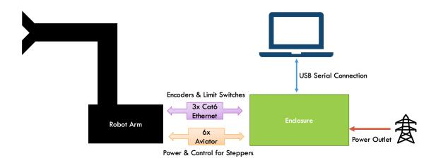
The enclosure has a standard computer power supply input, and this provides power to the stepper drivers inside. A computer running the AR4 Control program sends serial commands over the USB to the Teensy single board computer inside the enclosure. This is also how the Teensy receives its needed power.
