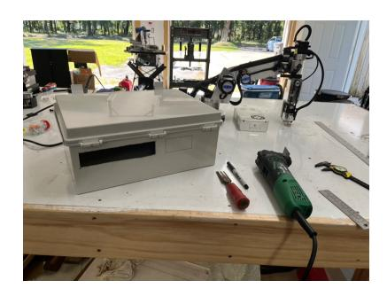
The holes are cut using an oscillating saw and the holes are drilled with electric drill.
