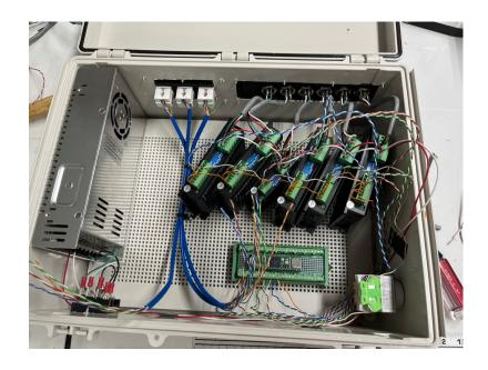
After double checking continuity and referencing the connection the schematic, the enclosure is now fully assembled.
