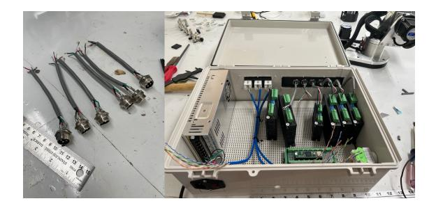
Starting with the power supply to the power outlet and continuing to emergency switch and the stepper drivers to the outside aviation connectors are wired.
