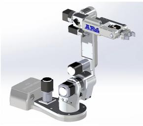
The AR4 is the fourth generation of the AR series robots. It includes a closed loop system with encoders built into the stepper motors as well as a 600MHz Teensy single board computer for on-board kinematics. The specification of this robot indicates that it expects to be able to deliver a 4lb payload with a repeatability of 0.2mm with a reach of 24.75 inches. [1]
